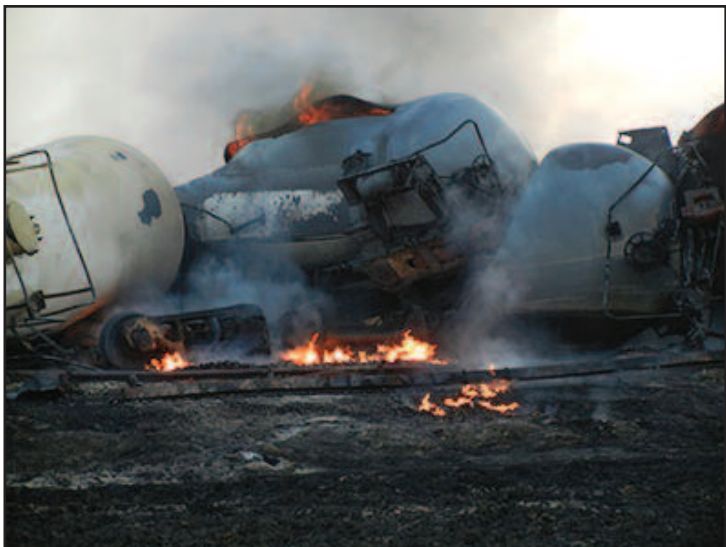
This photo, taken Dec. 31, 2013, shows part of the tank car pileup and residual fire resulting from the train collision near Casselton, N.D. The DOT-111 tank car in the center of the photo sustained a thermal tear, and is still burning. ©NTSB
