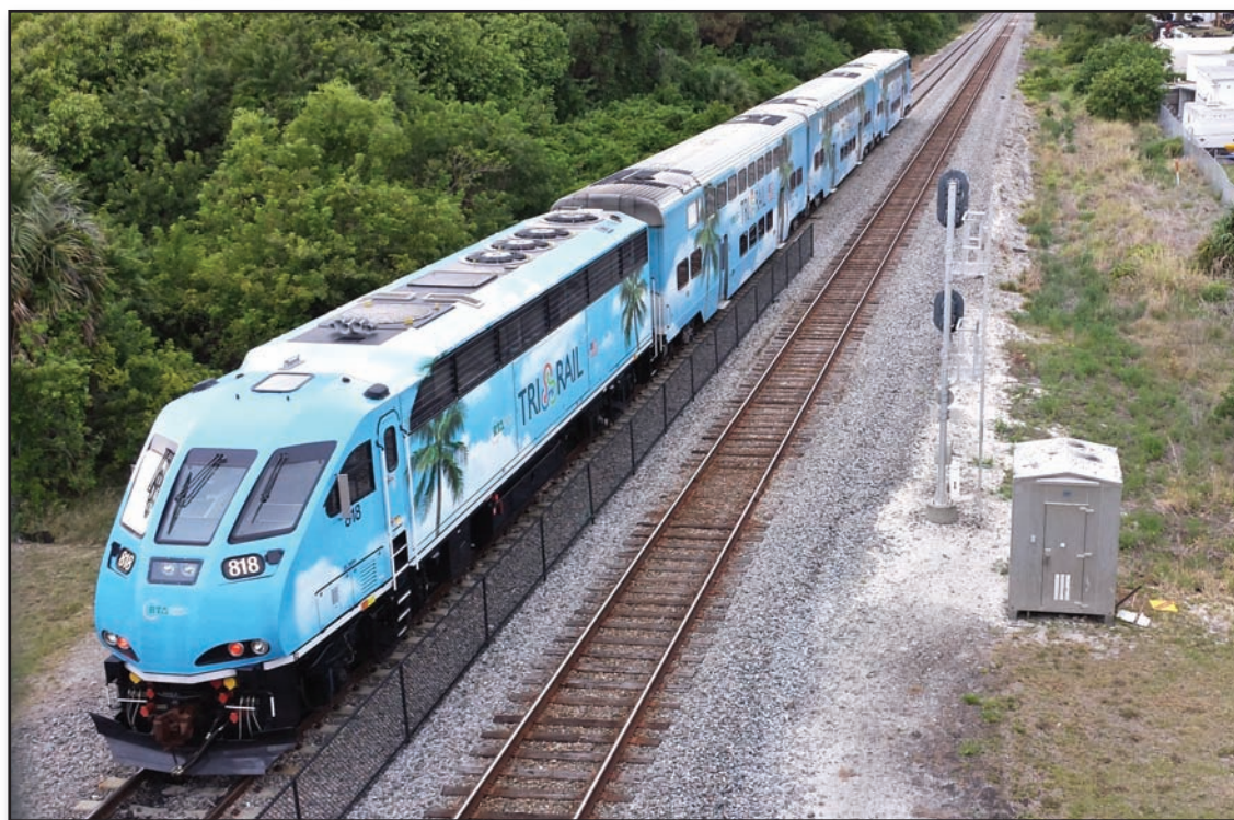
This photo was taken by Local Chairperson Andrew J. D'Egidio of Local 30 at Miami. "This is a picture of the new Tri-Rail Brookville BL36PH. The locomotive is built by Brookville Equipment Corp. specifically for Tri-Rail in South Florida and has a 3600 horsepower prime mover and a secondary Caterpillar diesel to provide head-end power. This is the first of 12 units delivered," D'Egidio said.
